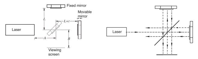
Figure 1: The Michelson interferometer. Left: equipment layout and distances. Right: ray paths. The offsets between ray paths are not real; they're just put in here for clarity.
