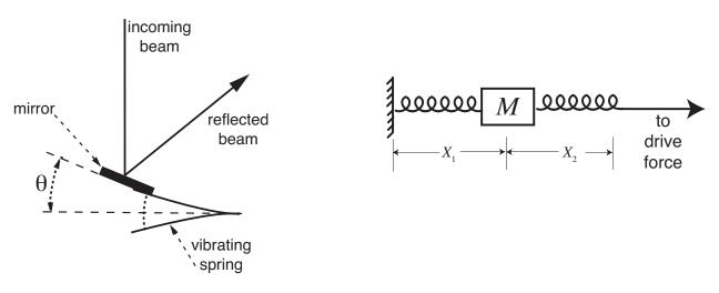
Figure 1: The left side is a schematic diagram of the vibrating sheet metal spring and the light beam reflecting from the mirror mounted on it. The right side shows the idealization of this oscillator as a mass-spring oscillator. The mass is at equilibrium at position  $x_1$  when it is at rest. Oscillations occur about  $x_1$  at the driving frequency  $\omega$  or, in the case of zero drive, at the resonant frequency  $\omega_0$ .
