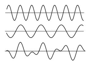
Figure 3: The upper two curves show oscillations at quite different frequencies with approximately equal amplitudes. Their sum is plotted in the bottom curve on a different scale. It is clear that the superposition motion of the sum shows no simple characteristics, and that its amplitude varies with time.
