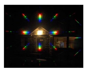
The spectrum of this light is not continuous, it has several discreet components. (A spectrum of better resolution could be obtained from a larger distance from the source.)
