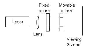
Figure 1: Schematic view of the Fabry-Perot Interferometer.
