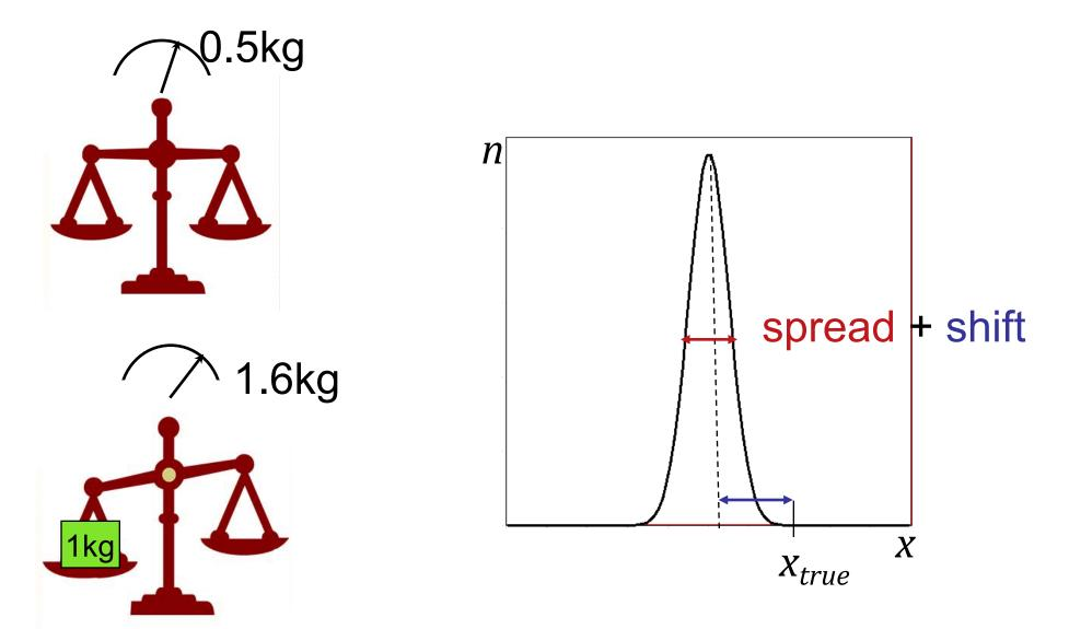
x can have a meaning of any measured quantity (e.g. box weight, acceleration due to gravity, etc)
