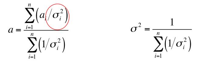
Each experiment is to be weighted by a factor  $1/\sigma_i$ . In this approach we do not check the degree to which  $a_i$  are mutually consistent.
