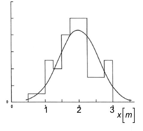
Continuous line is a known function (typically Gaussian) so called Probability Distribution Function (PDF)
