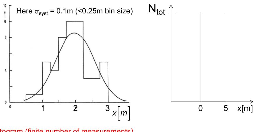
Histogram (finite number of measurements) Total number of measurments: N<sub>tot</sub> = N (bin1)+N (bin2)+ .... Function (infinite number of measurements)
