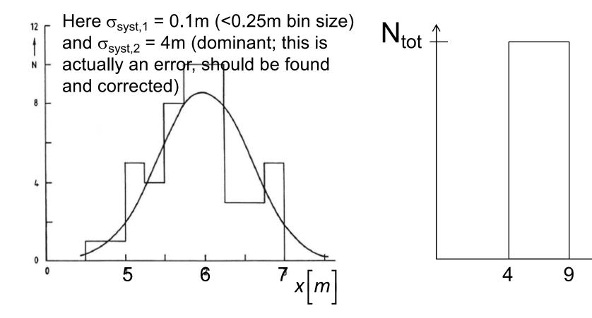
Histogram (finite number of measurements) Total number of measurments: N<sub>tot</sub> = N (bin1)+N (bin2)+ .... Function (infinite number of measurements) x[m]
