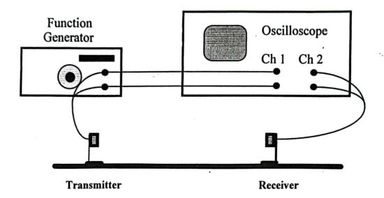
The function generator will be set to produce a square wave. Each rising or falling edge of the square wave will cause the piezoelectric transmitter crystal to "chirp" ultrasonically (in much the same way a hammer blow will make a bell ring). The function generator is wired to both the crystal and to the oscilloscope. The sound is received at a second crystal. A small amplifier is mounted to the receiver to make its signal large enough to be easily visible on the 'scope.
