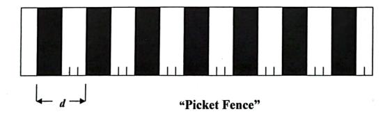
1. Measure the interval d between the two successive leading edges of the tape pieces; i.e., the width of one black strip plus one clear interval. To do this more accurately, measure the distance from the leading edge of the first black strip to the leading edge
